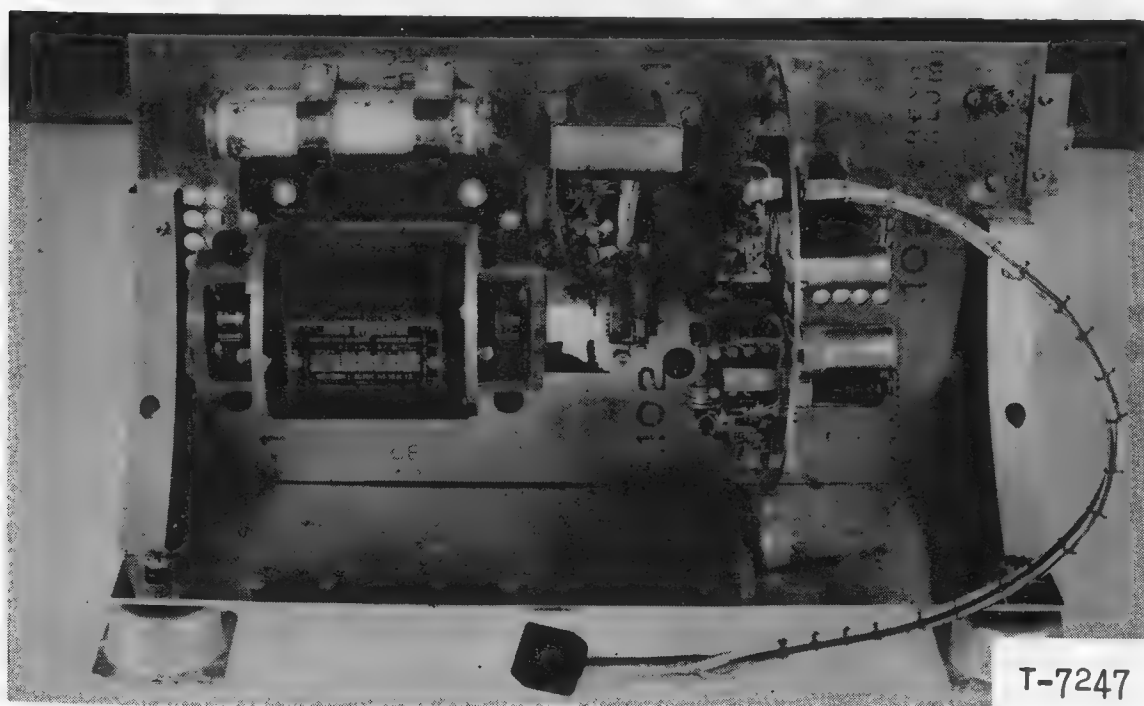
FIG 30 -- FINAL AMPLIFIER AND OSCILLATOR DECKS OF POSITION TRACKER TRANSMITTER
